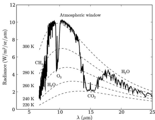
**Fig. 3.** Spectrum of terrestrial infrared radiation (Sportisse 2010). The spectrum is computed by the numerical model MODTRAN for the standard atmosphere (USA 1976, clear sky). The Planck black-body emission distributions are given for 220, 240, 260, 280 and 300 K. The corresponding greenhouse gases are indicated near the absorption peaks. This figure, from Sportisse (2010, fig. 2.12), is reproduced with permission © Springer.
